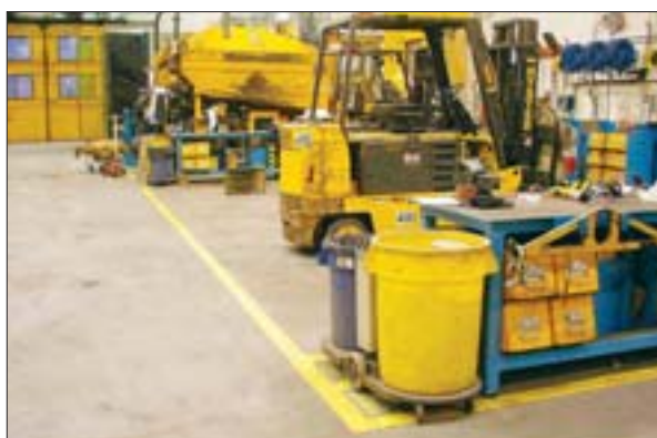
▲ Spill kits are located at the end of each work bench in the main garage.
