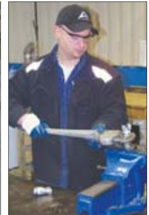
▲ Pipefitter Tony Fernandes puts together an air distribution T used to split air lines so they can be routed to different sections of the potroom.
