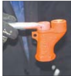
▲ A bronze Cleco air line valve from the potroom basements that has been rebuilt and repaired.
