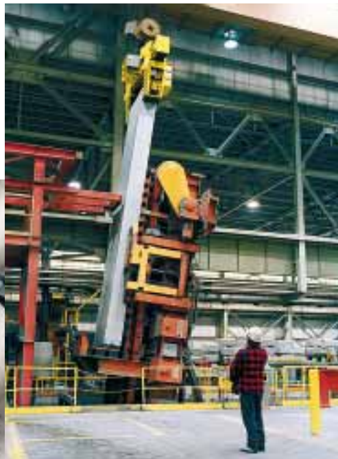
Sheet ingot emerging from casting pit
